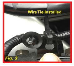
1) The "Christmas Tree" plug holding the defroster lines (fig. 1) is poking holes in the rear section near the bottom quarter panel seam of the top (fig. 2). This plug needs to be removed and replaced with a wire tie.
