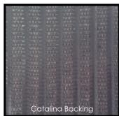
Catalina marine carpet features a ribbed vinyl backing designed for snapin installations.
